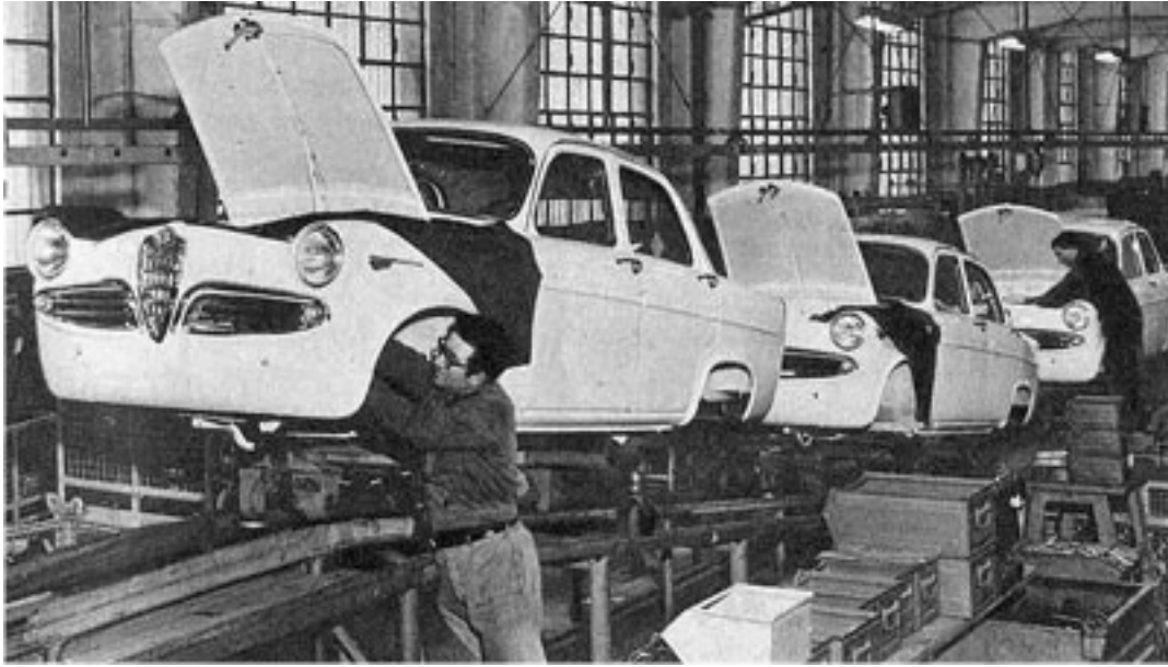
Installing the brakes and suspension.
