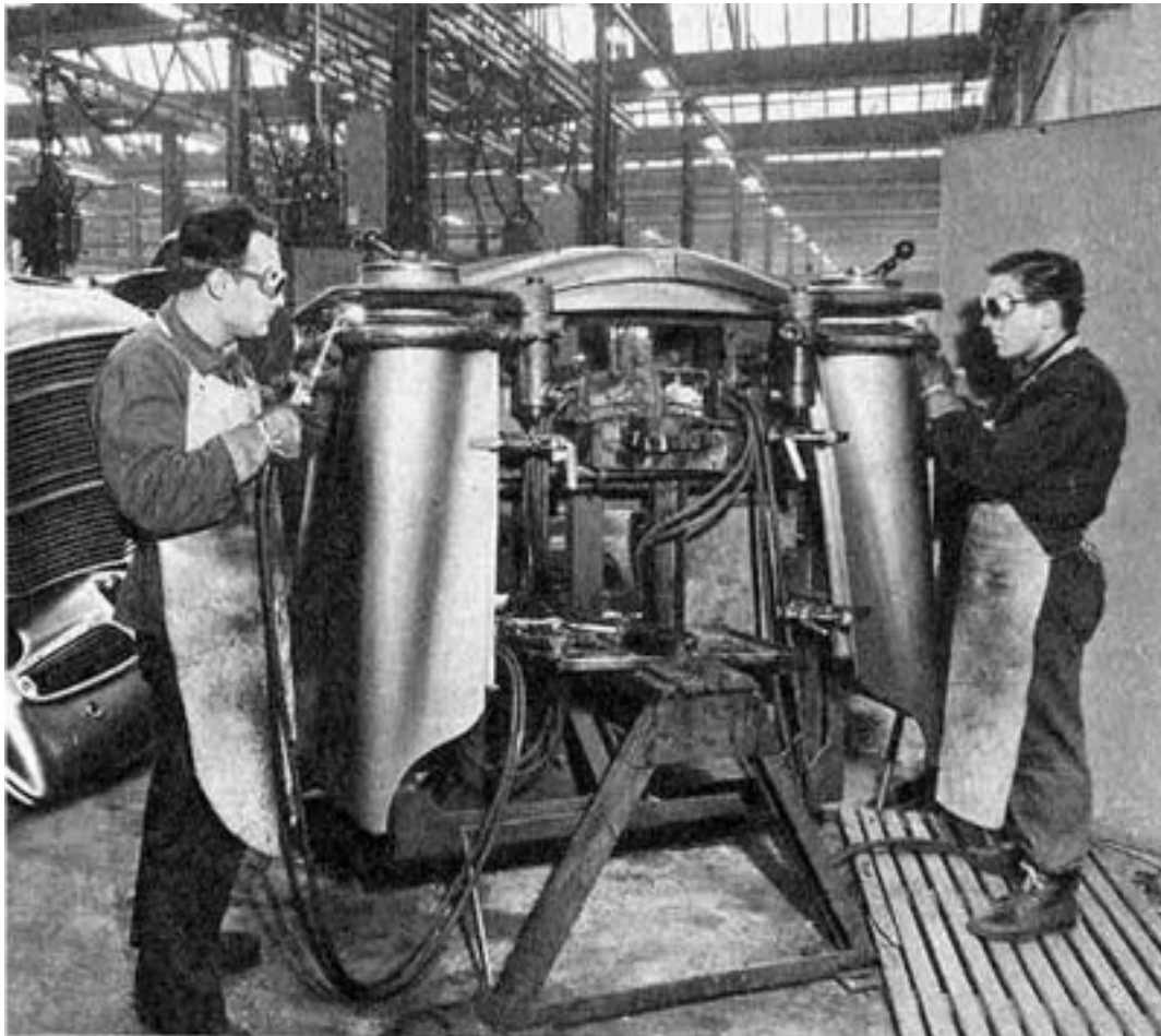
Front end of a Berlina is being welded together. While Alfa made the Berlina bodies, Pininfarina, Bertone and Touring constructed the Sprints, Spiders and 2600s in their own factories and shipped them to Portello for final assembly.
