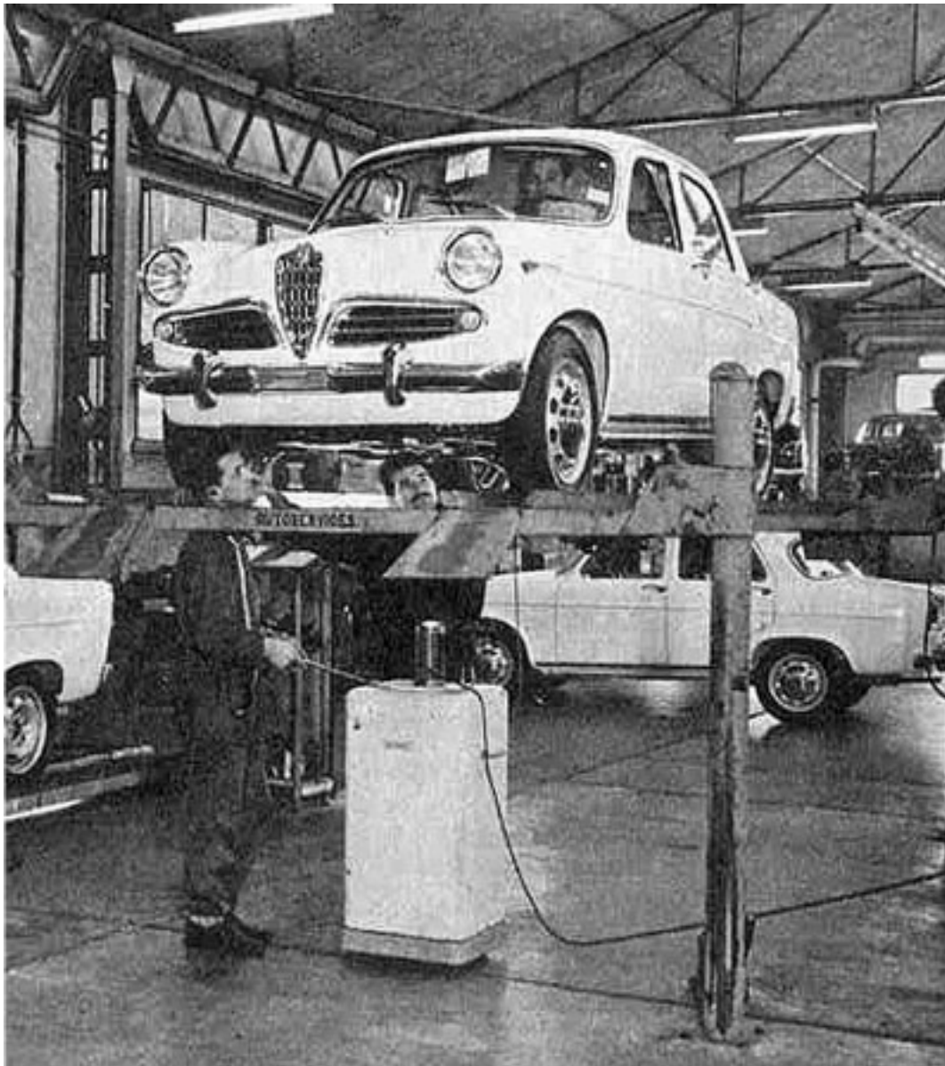
Checking and filling the fluids, the final step before testing each car.
